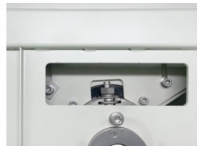
Stepless Adjustable Shaking Diameter
